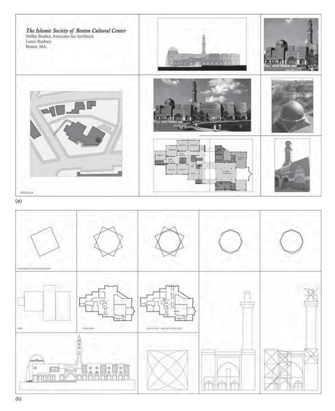
Figure 4.14 The Islamic Center of Boston: (a) formative concept; (b) analytic diagrams. (Site plan and graphics by Raheel Ahmed; photos by Muhammad Abdus Salaam)
